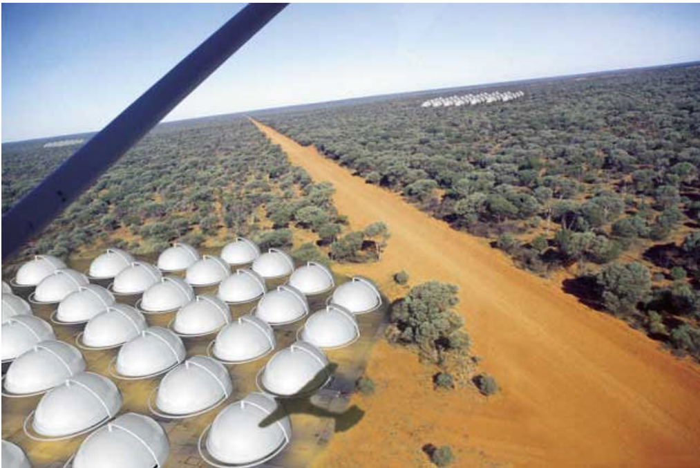
Figure 3: Artist's impression of SKA stations composed of 5m diameter Luneburg lenses
