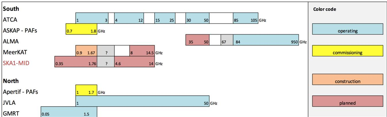
Figure 2: ATCA frequency coverage compared to other radio synthesis arrays (details in Table 1).
