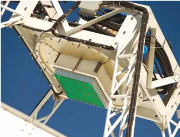
A prototype of ASKAP's phased array feed (or 'radio camera') technology on the 12-metre antenna at the Parkes Testbed Facility, which is used for testing ASKAP's systems. Image Credit: David McClenaghan, CSIRO.
