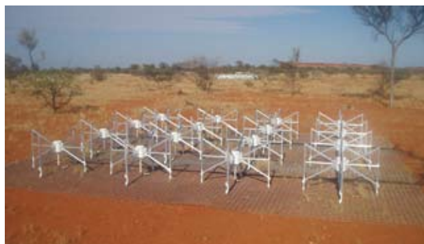
An MWA tile in the field, showing the ground-plane and the 16 dipoles (Photo Credit: Steven Tingay).
