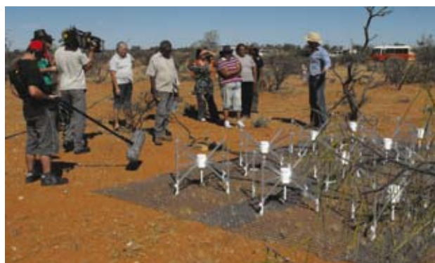
While touring the Murchison Radio-astronomy Observatory site, the group visited one of the MWA tiles (an installation of 16 dipoles). Photo Credit: Megan Argo, Curtin University of Technology.
