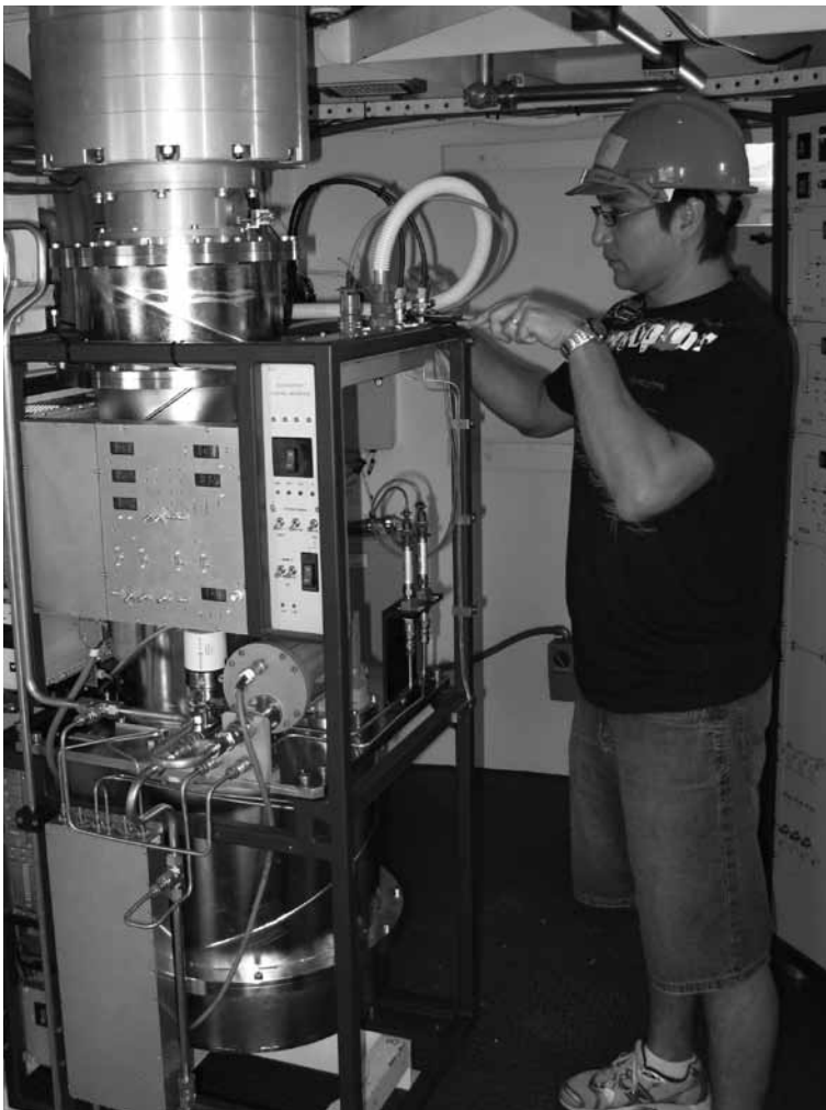
Santiago Castillo installing an upgraded 1 – 3 GHz receiver system. Credit: Henry Kanoniuk, CSIRO.
