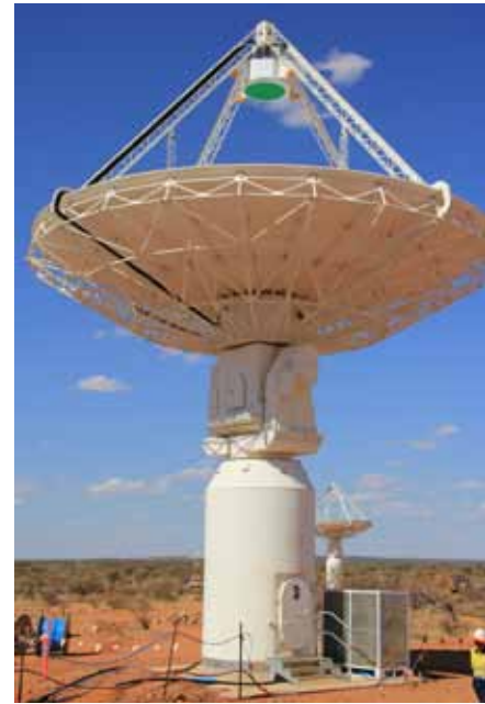
The first full-sized phased array feed receiver was installed on an ASKAP antenna at the MRO in October 2011. Credit: Image courtesy of DIISRTE.
