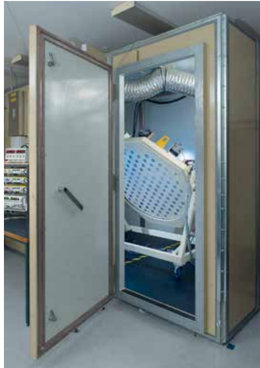
The prototype Mk II PAF set up in the SKA Lab, an RF-shielded room at CASS headquarters in Sydney. During the tests all 188 RF signals were successfully transported from the PAF to the digital backend, located in an adjacent room.
