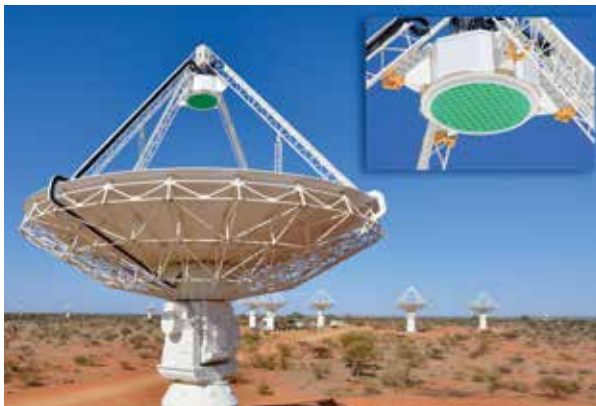
A close-up of a phased array feed (PAF) receiver installed on an ASKAP antenna at the Murchison Radio-astronomy Observatory. Following the successful installation of the first six PAFs at the MRO, commissioning activities are now underway with the engineering test array, ‘BETA’.
