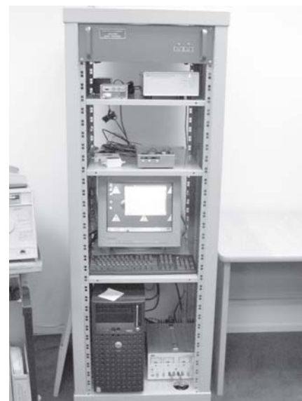
Figure 1: The downconversion system, receiver, clocks, and recording system developed by Tim Natusch at the Auckland University of Technology.
