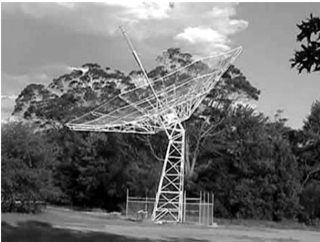
Figure 5: One of the old Culgoora heliograph dishes. This is one of an array of 96, 13.7-m dishes that circled the present location of the Compact Array. The heliograph array imaged the Sun at 80 and 160 MHz with several discoveries to its credit.
