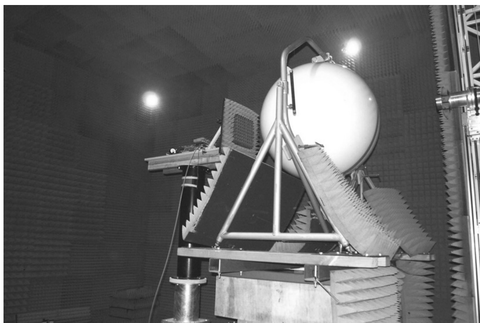
Figure 1: Luneburg lens and focal plane array being tested in the CSIRO near-field test facility.
