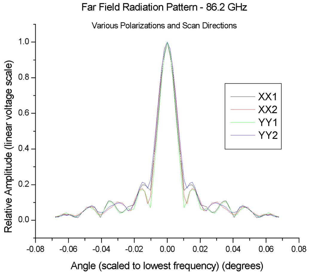
**Figure 4 :** Beam patterns for the two cross scans and in the XX and YY polarizations; all at 86.2 GHz.
