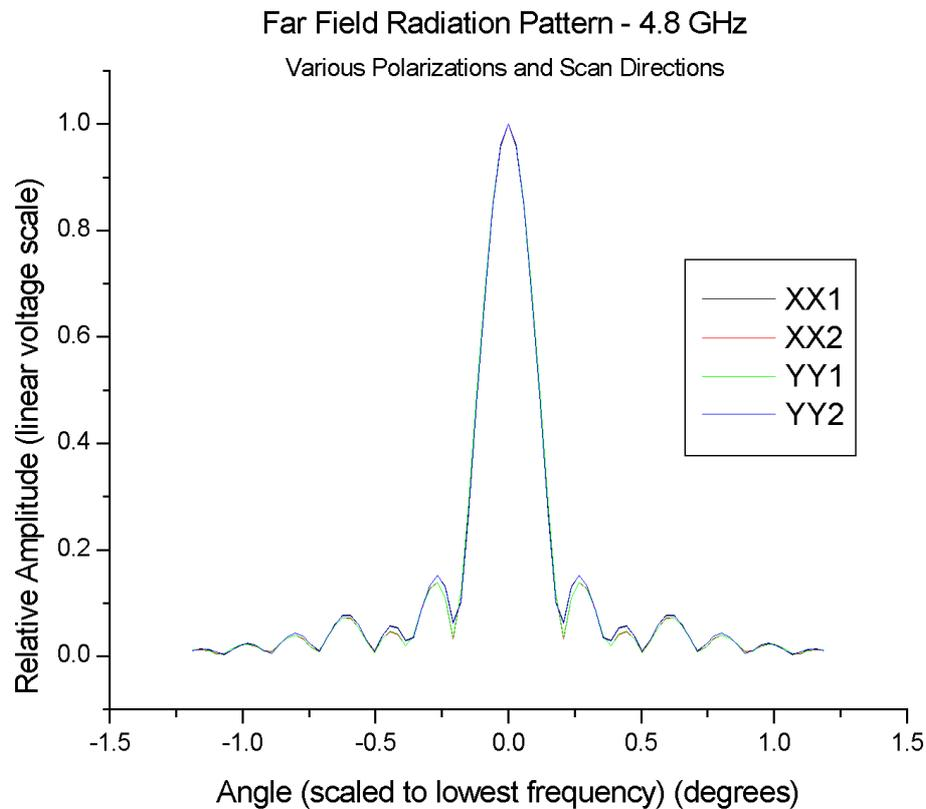
**Figure 3 :** Beam patterns for the two cross scans and in the XX and YY polarizations; all at 4.8 GHz.
