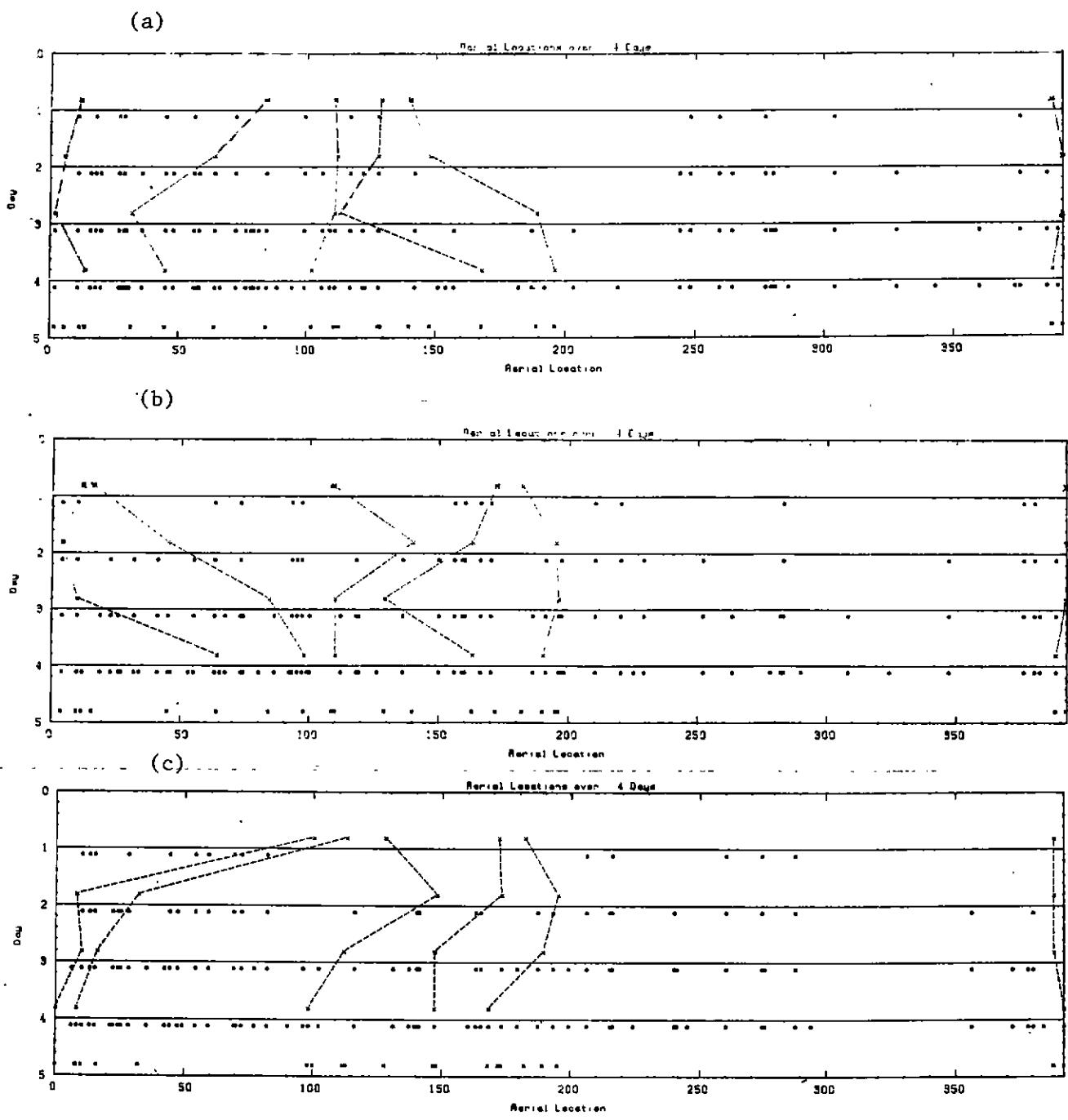
Fig. 3.7 : Antenna locations and baseline distributions for the three individual 4-day segments of the optimized 6km array (Fig. 3.5); (a) days 1-4; (b) days 5-8; (c) days 9-12.
