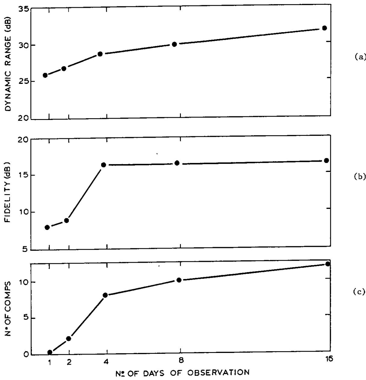
Fig. 5.5 : Dynamic range, map fidelity (see text for definition) and number of clearly identifiable weak components in CLEANed images of SPIRAL as a function of number of days of observation with the 3km array. The source components were counted from the one at  $(l,m)=(-140,-40)$ . (See Fig. 5.1.)
