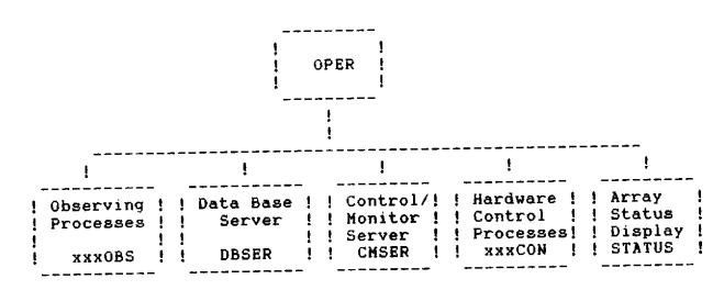
OPER: Provides the operator interface to the AT. It initiates and controls all other processes.
