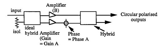
By varying the gain of the A channel, relative to that of the B channel, the isolation between the circular polarised outputs may be measured.
