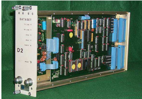
Figure 3.2: A photo of a “D2” dataset module. These units have provided sterling service to the Compact Array since their design in the 1980s. Parts for these modules are becoming increasingly scarce as they reach the end of their design life.
