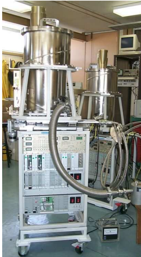
Figure 1.2: Two Compact Array millimetre receiver prototypes, undergoing cool down tests in the Narrabri receiver workshop. Much of the ancillary equipment, such as the down conversion modules and Water Vapour Radiometer, are missing in this picture.
