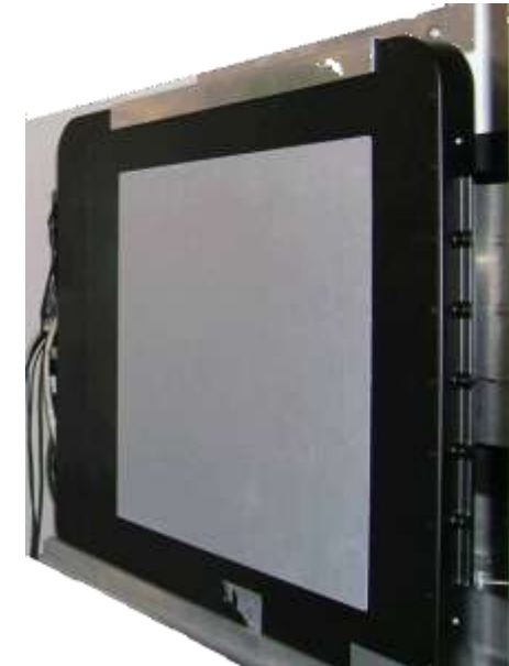
A 2k x 2k 16-bit panel kindly lent to us by PerkinElmer, later purchased.
