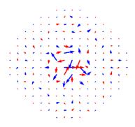
Beamformer weights for a central beam (colours represent polarisations), created using the new software service
