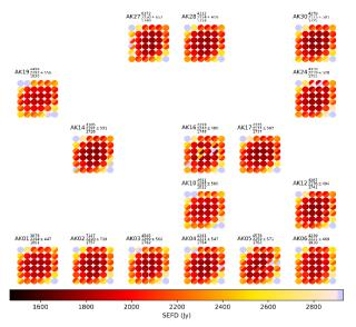
Plot showing an SEFD test where all beams on 16 active antennas have been measured. This shows the consistency of beams formed on all antennas. Similar observations with different beam spacings can be used to determine FoV.
