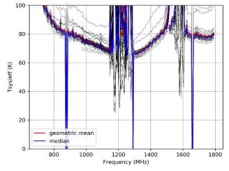
ASKAP system temperature as a function of frequency for a single boresight beam, made using 5 different frequency tunings over the three available filters. Each antenna is shown as a thin back line, with the mean and median in red and blue.
