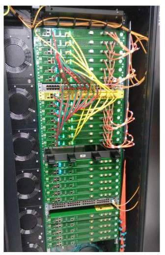
One of the complete correlator blocks (top) and a partiallyinstalled block below.
