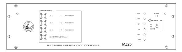
Test points for the D.C supplies are available on the front panel.
