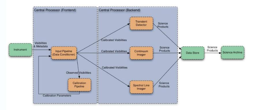
Data from same set of visibilities can be passed through three pipelines for **Transient, Continuum** and **Spectral Line** imaging.
