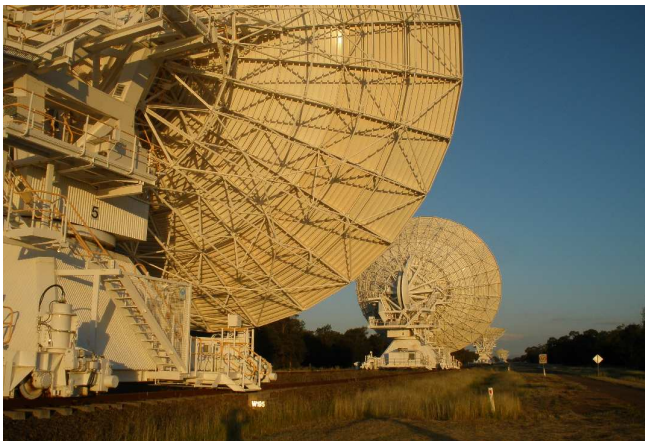
Figure 2. The Australia Telescope Compact Array (ATCA). Displayed are several antennas on the East-West track pointing at a source near the horizon.
