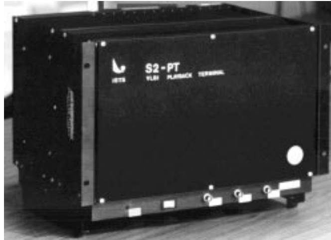
Figure 1-2: Data, Signal and Control Module (DSCM)
