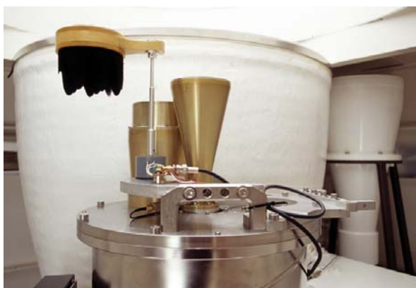
One of the new prototype receivers, in the upper vertex room of antenna 2, installed next to a large white 20-cm feed horn. The feed horn for the 12-mm waveband is in front of the 3-mm waveband (installed inside a vacuum dewar). A radio frequency absorber paddle can be seen above the two horns.
