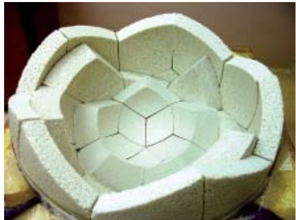
A trial assembly of the Luneburg lens components. Photo: © CSIRO
