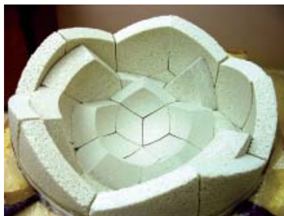
A trial assembly of the Luneburg lens components. Photo: © CSIRO
