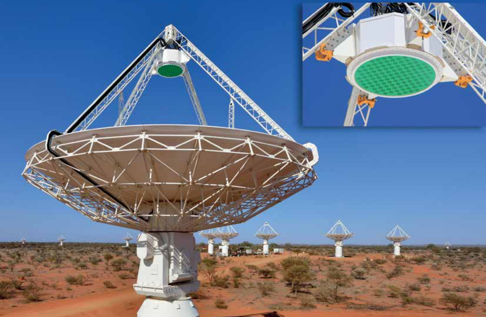
A close-up of a phased array feed (PAF) on an ASKAP antenna — one of the first six PAFs successfully installed this year.
