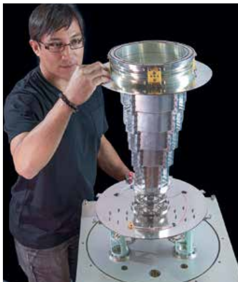
CASS receiver engineer Santiago Castillo, with the CASS-designed feed proposed for China's FAST telescope. Credit: Wheeler Studios
