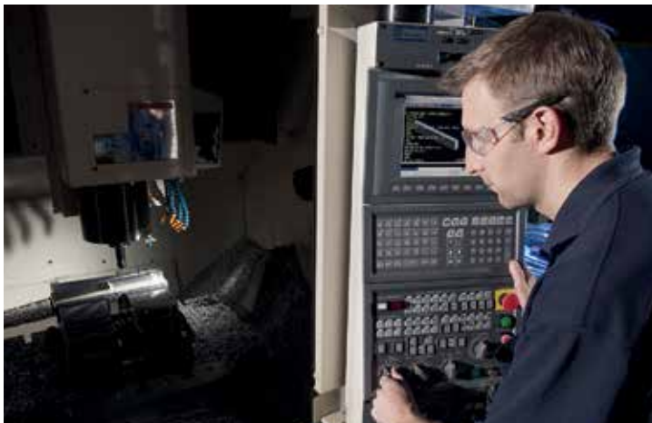
CASS technical officer Michael Bourne machining a new orthomode transducer for the Compact Array. Credit: Wheeler Studios
