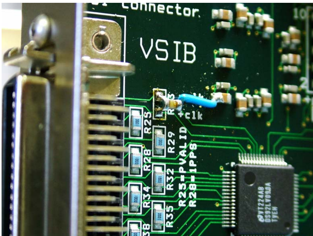
Photo 3 - Close-Up View Of Clock Termination Modification Showing "Tombstoning" Of Split Termination Resistors
