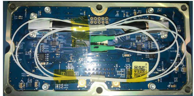
Figure 8. Photograph of the optical transmitter layer in the domino, referred to elsewhere as TRANSMITTER.
