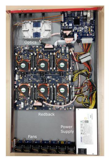
Image: Top-down view of a beamformer chassis with the cover removed to show the components described above.
