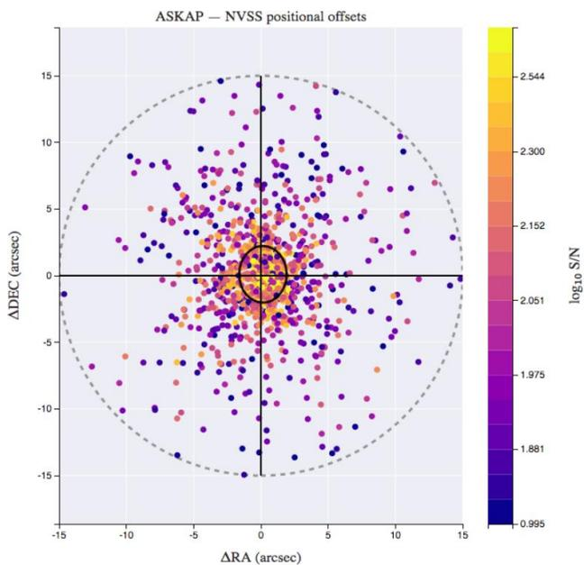
Plot of source position offsets with respect to NVSS from a recent ASKAP image after delay tracking improvements
