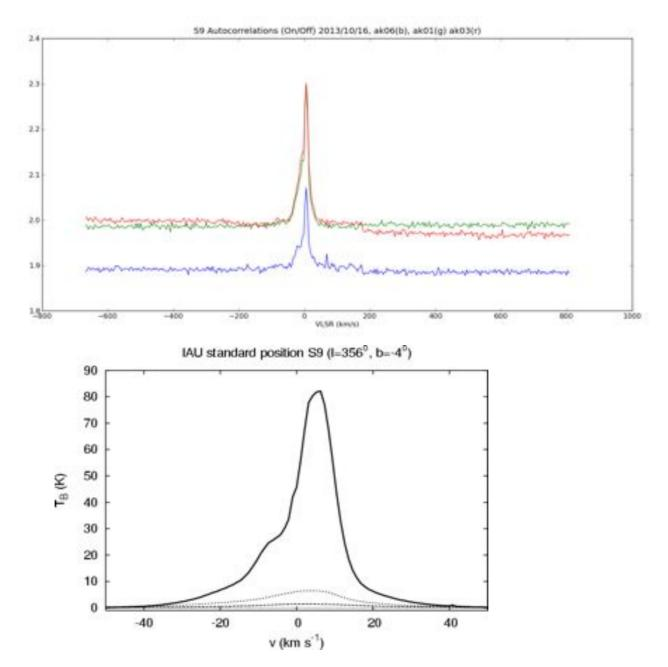
Figure 1 (Top): Autocorrelation spectra from observations of a Galactic region of neutral hydrogen IAU S9 using ASKAP antennas 1,3 and 6 (green, red, blue). The xscale is velocity relative to the local standard of rest and the y-scale is the ratio between on-source and off-source Tsys. Bottom: Reference spectrum from Bajaja et al. (2005) showing the line profile.
