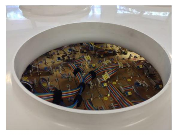
*Figure 2: Prototype Mk II phased array feed undergoing integration tests at the Marsfield labs.*
