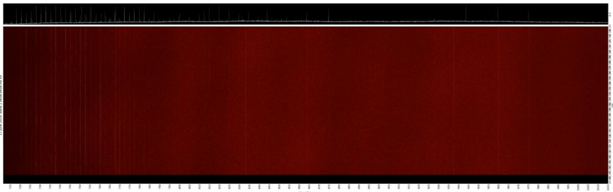
Figure 7: Frequency-time visibility plot showing very low levels of RFI in a typical observation in the 700-1000 MHz band using BETA. The 'comb' of narrow features (left) originates from the BETA cooling system. This will not be present in the ASKAP spectrum. Credit: Lisa Harvey-Smith, Balt Indermuehle/ACES team, CSIRO.
