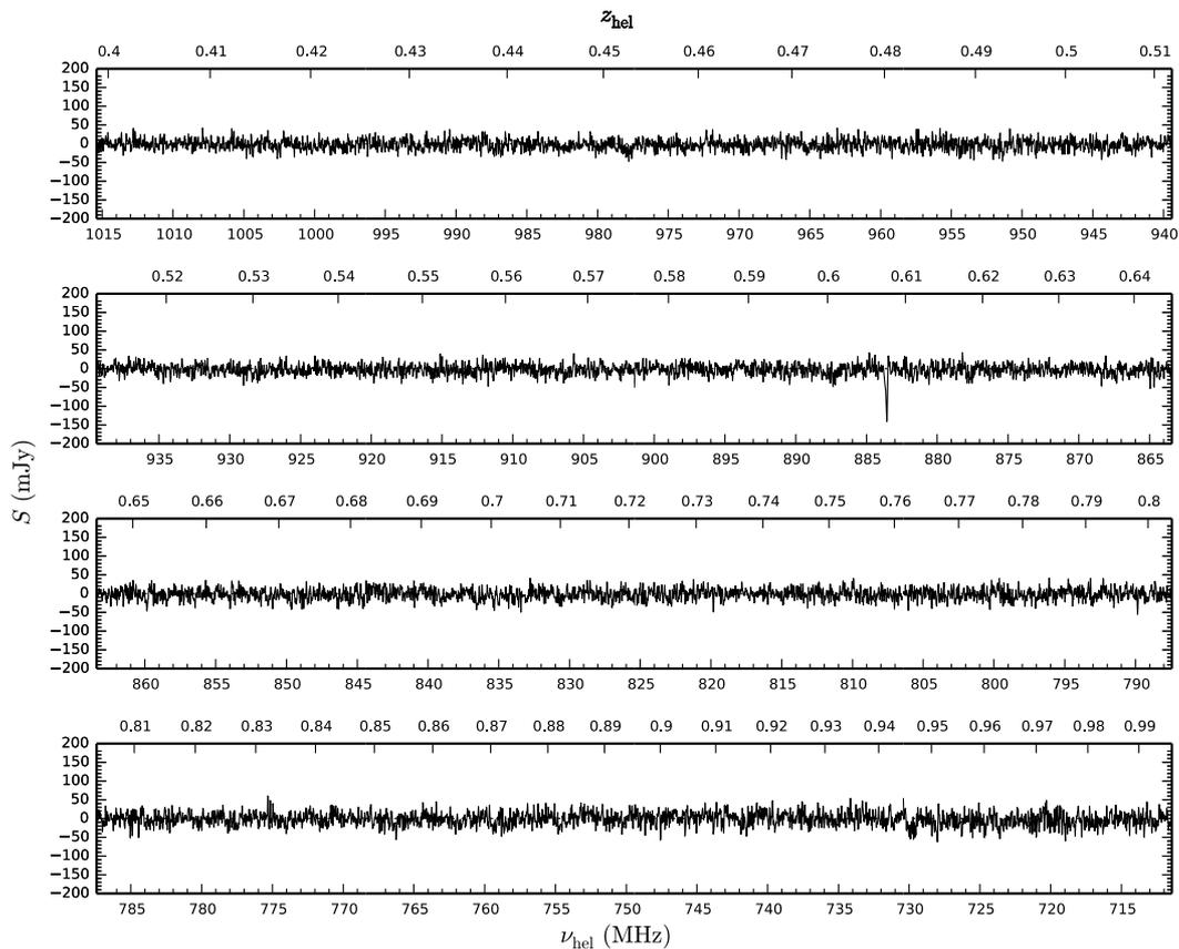
*Figure 3: Spectrum towards the 1Jy radio galaxy PKS2252-089 taken with BETA. The known intrinsic HI absorption line can be seen at 884MHz. The data have been automatically flagged for birdies and other narrow-band RFI, and further Hanning smoothed to improve the visibility of the HI line. The noise rises slightly towards the lower frequency end of this spectrum as expected. Credit: James Allison/ACES team, CSIRO.*
