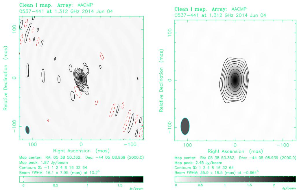
*Figure 9: Total intensity image of 0537-441 using the Australian Long Baseline Array, (left) with a single ASKAP antenna and (right) without ASKAP. Credit: Chris Phillips, CSIRO.*
