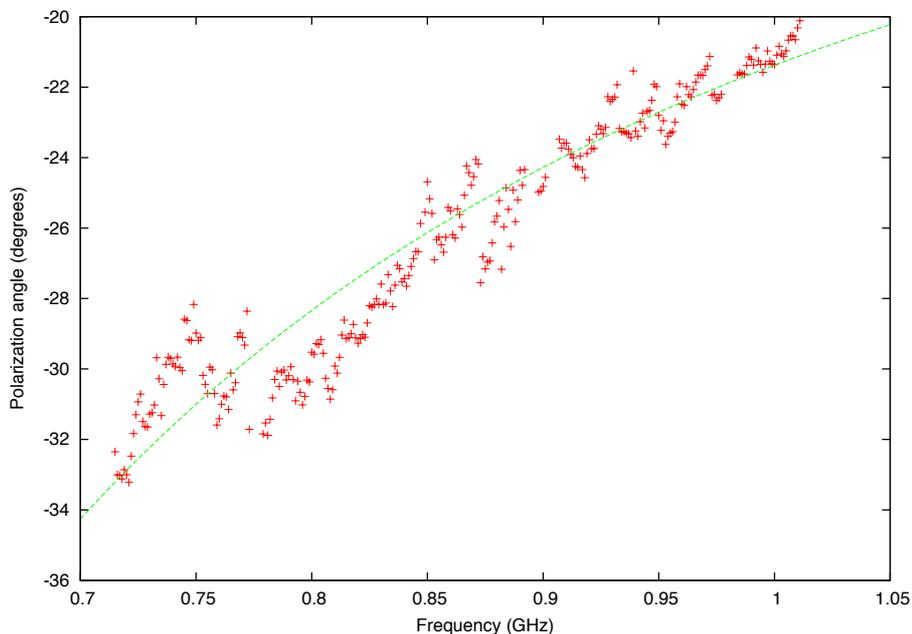
*Figure 4: Measured frequency variation of the polarisation position angle of 3C138 (symbols) and a model fit. Credit: Bob Sault/ACES team, CSIRO.*
