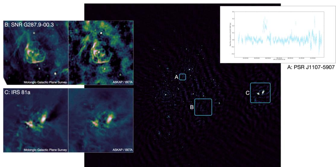
*Figure 1: BETA image from a single beam showing a region of the Galactic plane and the light-curve of a variable pulsar derived simultaneously from the data. It was made from 13 hours of data between 0.7 – 1 GHz. Credit: I Heywood/ACES team, CSIRO.*
