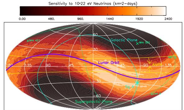
Figure 6: Likely sensitivity ( $\text{km}^2\text{-days}$ ) to  $10^{22}$  eV neutrinos ASKAP in celestial coordinates for one month's observations (40% duty cycle). A frequency band of 0.7–1 GHz is assumed. The sky coverage is much broader than for ANITA Antarctic ice balloon experiment (Miocinovic et al. 2005).
