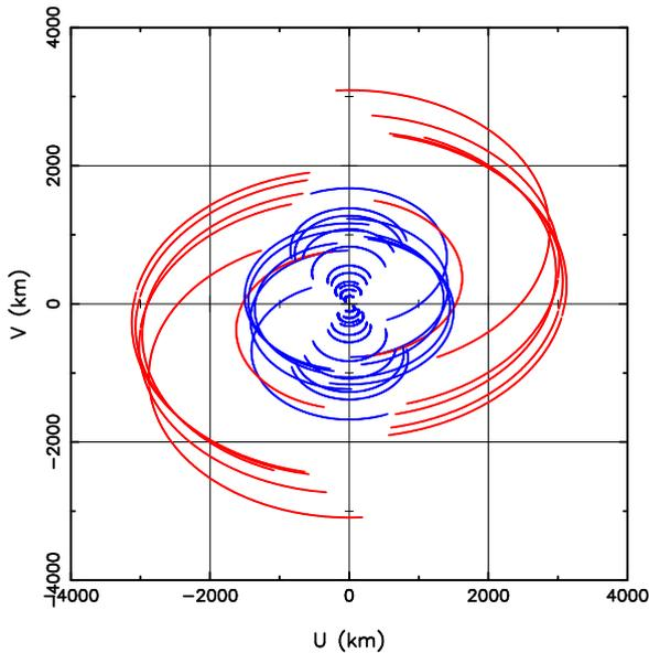
Figure 4: The  $(u,v)$  coverage of the current Australian VLBI array at 1.6 GHz (blue curves) and with the inclusion of ASKAP (blue and red curves combined). The improvements in the east-west component of the baseline distribution and in the extension of the maximum baseline length are significant.
