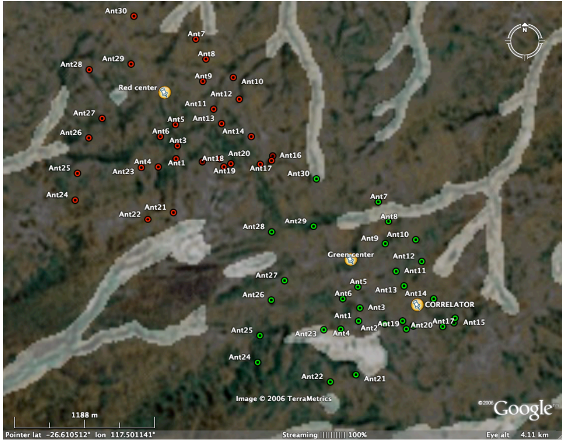
Figure 7 XNTD30 RED and GREEN - 30 12m diameter antennas giving 30 arcsecond resolution for a 300MHz band with upper frequency 1.4GHz
