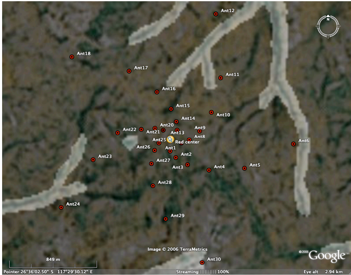
Figure 10 XNTD30SPIRAL/RED - Spiral armed array with 30 arcsecond resolution
