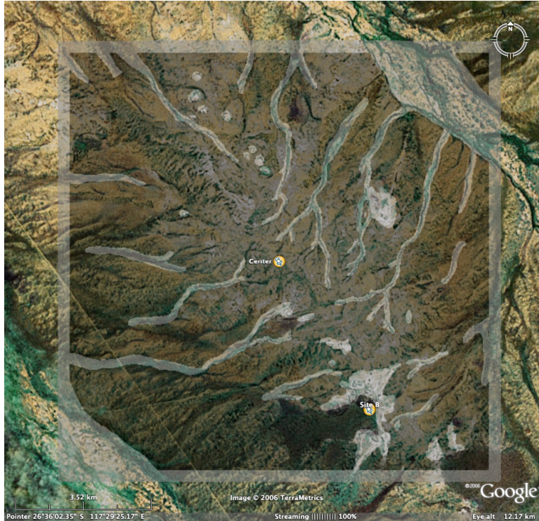
Figure 5 Environment constraints (from Holm and Associates, 2005) superimposed on Google map. Light areas are not to be used for antenna sites. The enclosing green box is 10,800m across (inside edges), and spans 500 pixels in the mask image.
