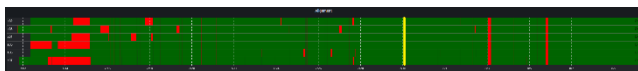
Figure 1: Colour-coded monitoring data from ASKAP’s control system showing fewer unexpected alignment failures (red blocks) after the test firmware deployment. Date increases to the right for one month, ending on the 9 th of August. The new firmware was deployed at the yellow line. Red lines at full height are intentional resets or system downtime.
