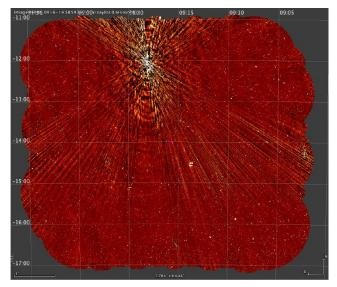
Figure 1: Pipeline image of an EMU field containing Hydra A, showing significant artefacts. Image supplied by Emil Lenc.
