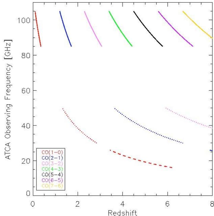
*High Redshift CO windows accessible to the ATCA with the 3 mm (solid line), 7 mm (dotted lines) and 12 mm (dashed lines) systems. These correspond to the three bands on the y-axis, from 85-105, 30-50 and 16-25 GHz, respectively. CO transitions start from  $J=1-0$  at the left, and increase (i.e. 2-1, 3-2 etc) with redshift.*
