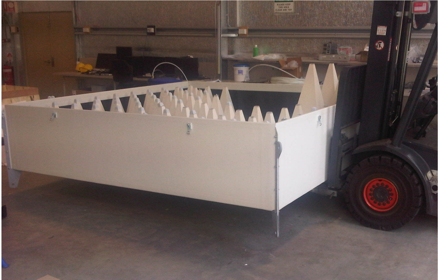
Hot load for ADE PAF ground tests en route to MRO
