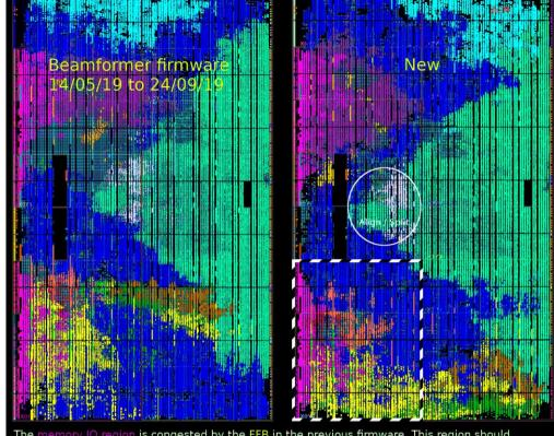
The memory IO region is congested by the FFB in the previous firmware. This region should and the pre+post buffers. In the latest firmware the FFB moves away from this critical region down to the bottom. The Fringe rotator and anti-ripple modules also follow. The patterned box has been added as a pblock (floorplanning) to keep the memory arbiter and pre/post bufferrs close to the memory IO. Others: ACM, Inter FPGA Alignment, Beamformer Engine
