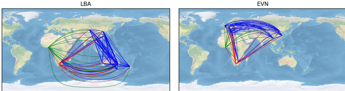
Figure 8: Geographic locations of radio telescopes that could be used to form a VLBI array with SKA1-MID. (left) **LBA**: Baselines to MeerKAT (red), an African VLBI station in Ghana (green), and an extended LBA array with some Asian telescopes (blue); (right) **EVN**: Baselines between MeerKAT (red), Ghana (green) and the northern-hemisphere EVN.
