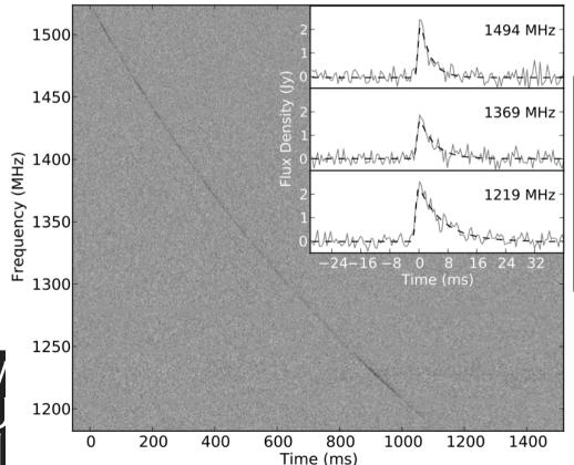
Bright enough to fit the pulse shape as a fn. of frequency to find dispersion & scattering indices
