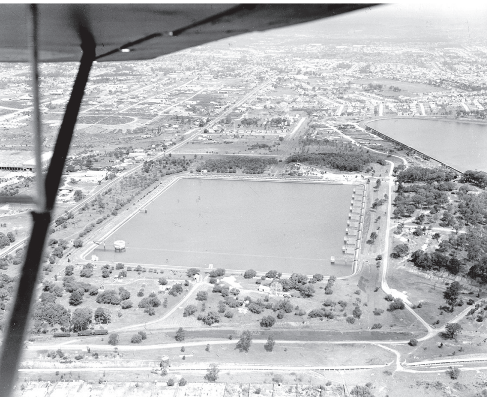
Figure 1: An aerial photograph of Potts Hill field station taken on 19 March 1954. The view is from the north looking south. The main part of the field station is in the immediate foreground. The East-West solar grating array is on the southern bank of the reservoir and the North-South array on the eastern bank. On the bottom left, three coal train carriages are visible. These were used to supply coal for the steam driven pumping station for the water supply reservoir. The main road visible on the left is Rookwood Road.
