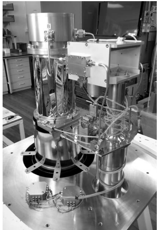
Photo of the retrofitted L/S receiver with new amplifier in place. Credit: Eliane Hakvoort, CSIRO
