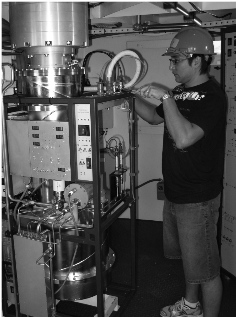
Santiago Castillo installing an upgraded 1 – 3 GHz receiver system. Credit: Henry Kanoniuk, CSIRO.
