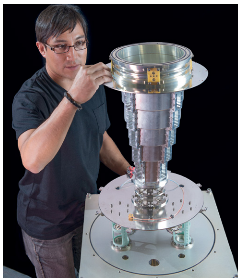
ATNF receiver engineer Santiago Castillo, with the CASS-designed feed for China's FAST telescope. Photo: Tim Wheeler
