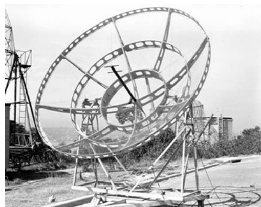
Figure 3: One of the simple 3-m diameter alt-azimuth-mounted “solar eclipse” antennas undergoing testing at Georges Heights in August 1948 (ATNF Historic Photographic Archive: B1511).
