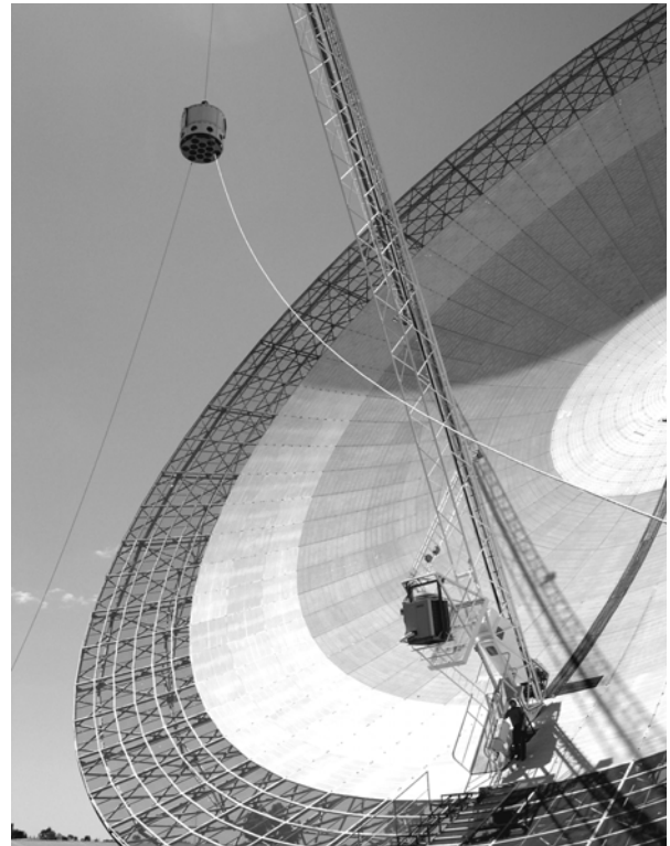
Figure 1: The Parkes multibeam receiver being removed from the focus cabin on 22 October last year. David Catlin can be seen working the hoist.
