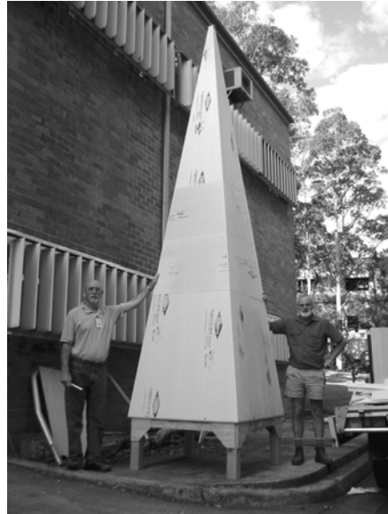
Figure 1: Barry Parsons and Michael McDonald with their creation: the styrofoam structure of the pyramidal antenna. The three-piece pyramid was built in the Marsfield workshop by gluing together precisely cut styrofoam slabs.
